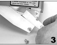
Carefully remove knife shim, set aside.
