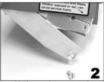
Extend knife cover down to expose internal blade components.
