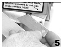
Next, remove spacer from knife block as shown and set aside.
