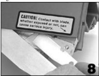
Reinstall knife shim over spacer. Slide cover back and insert screw.
