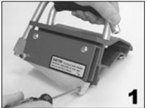
Steady tool on flat surface. Extend knife block and remove slotted screw.
