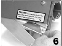
Reinstall blade into knife block using the first alignment notch on blade.
