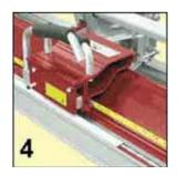
**4. Automatic** After separation, material is automatically set for standard 3/4" bend, or true 180 degree hem.
