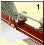
1. Score Entire Length Lock material in brake at desired width + 3/4". Extend QuickScore<sup>™</sup> along entire length of material.
