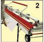
**2. Press Downward** Extend material downward along score. Use uniform pressure to avoid kinks.
